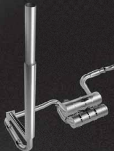
NEW UNDER-CAB VERTICAL SWITCHBACK exhaust system is a compact option with pipe routing similar to the "big rigs" exiting at the top of the cab on the passenger side.
