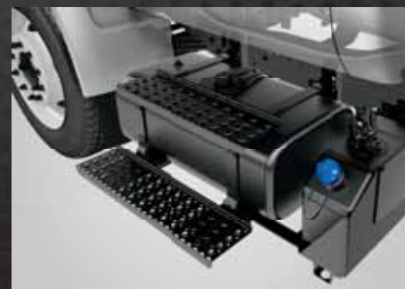
NEW 35-GAL. FUEL TANK and 5-GAL. DEF TANK option mounts under the cab on the driver's side for a Clean CA on Regular Cab models.
